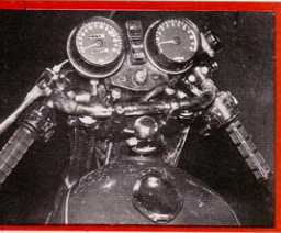
The cut and welded bars created by Dave Walker. The right bar was damaged in a minor incident early on in the test.
