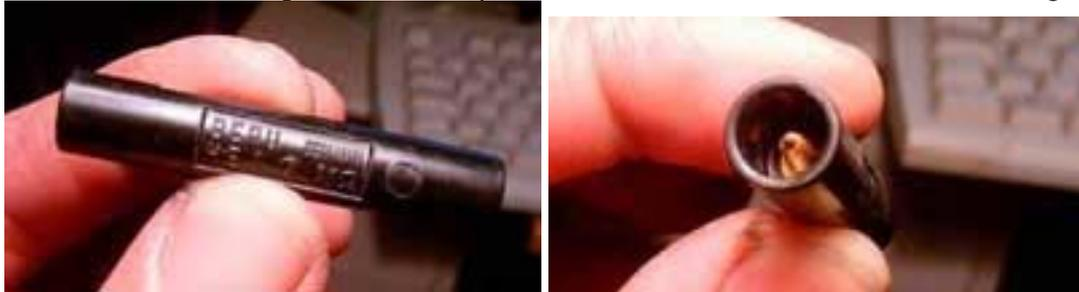
Cut the wires and screw the cable ends into the resistor tube. Pull a heat-shrink tube over each of the resistor tubes and shrink them. They should be a little longer than the resistor tube to be able to make a waterproof seal.
